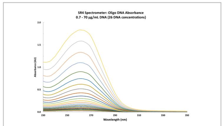
Even a small amount of protein contamination in DNA solution can have a large effect on UV absorbance. In this case, the SR4 demonstrated good linearity up to 2 AU.
