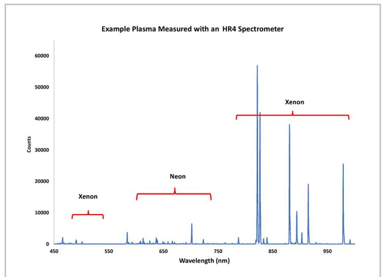
As a high-resolution, thermally stable spectrometer, the HR4 is ideal for monitoring the emission peaks of gases used in semiconductor and other manufacturing processes.
